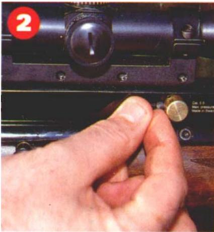
Place a pellet in magazine port and release magazine.
