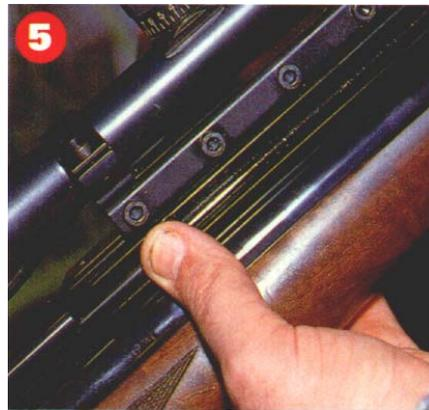
With magazine **STILL PUSHED FIRMLY TO THE RIGHT**, close the bolt.
