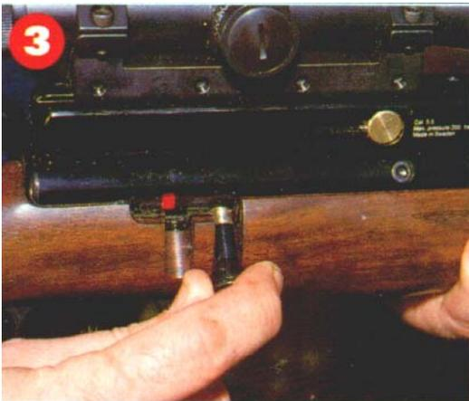
Seat the pellet into the bore by pushing the bolt forward, then draw back the bolt once again.
